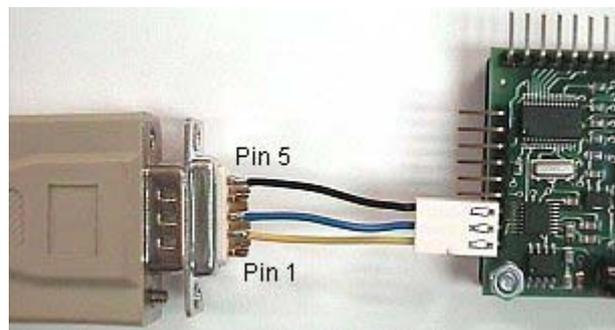
The serial data format is 8bits, No Parity, 2 stop bits, 38400 baud.
