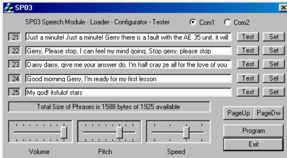
When you run the program for the first time, you should select the communications port you will be using, either COM1 or COM2. This will be remembered for the next time you run the program.
